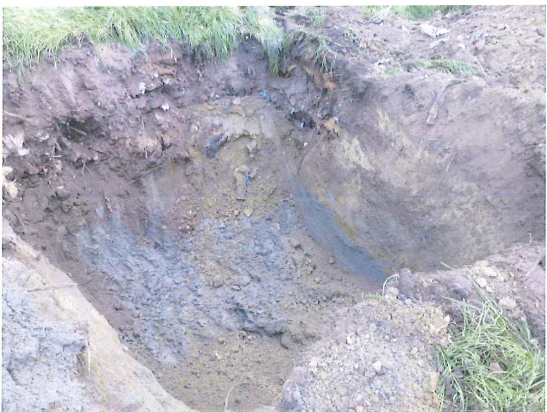
*Photograph 2: Test pit 3 – edge of old waste pit*
